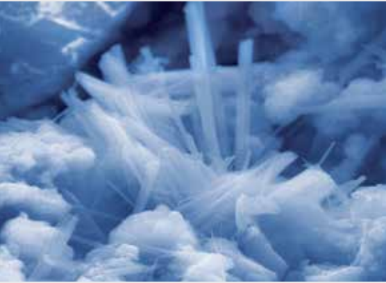
PENETRON active ingredients react with concrete minerals to form insoluble crystals, which fill in cracks, pores and voids up to a width of 500 microns (0.5 mm). (Magnification 5,000x)
